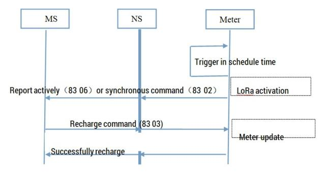
Remark: Recharge key information use DES encryption, fill the user number at the first time to recharge and complete the binding between user and meter; Check the user no. and times of gas purchasing in the follow-up recharge process, only if the times of gas purchasing in the recharge information is more than 1 time comparing with the times in the gas meter, the system judge the recharge information is valid.
